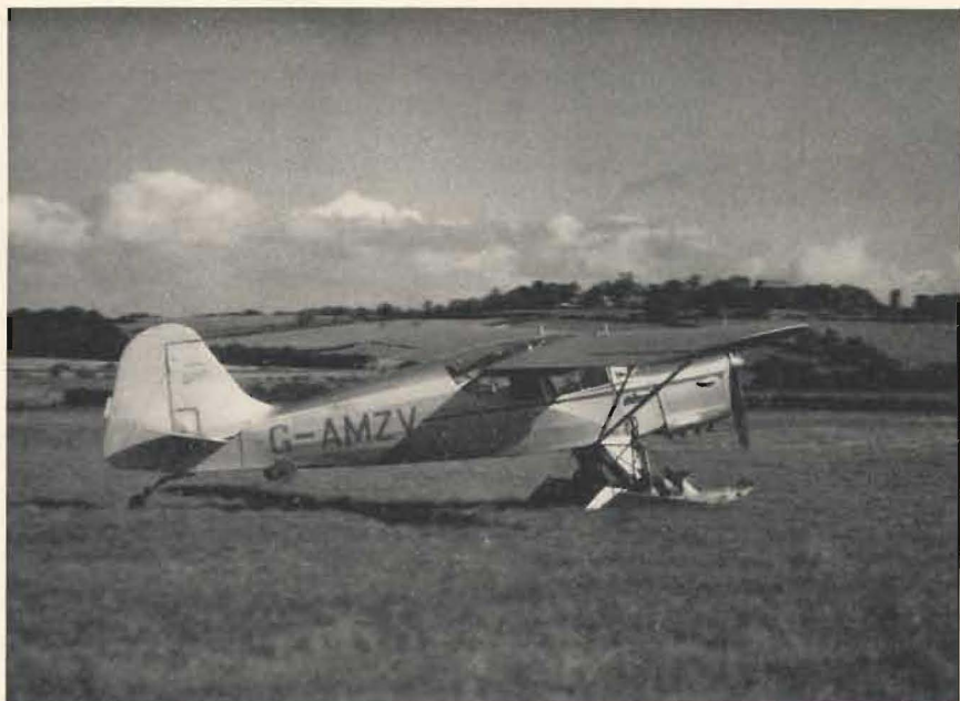
Take-off from land is also possible as the main wheels protrude through the skis.
